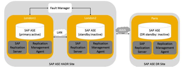
The HADR with DR node system includes an embedded SAP Replication Server, which synchronizes the databases among three servers. The system uses Replication Management Agent (RMA) to perform the initial setup and HADR operations.
